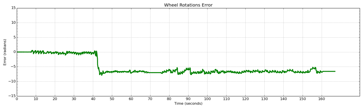
Figure 14: Drift in Estimated wheel rotation with respect to Ground truth data
