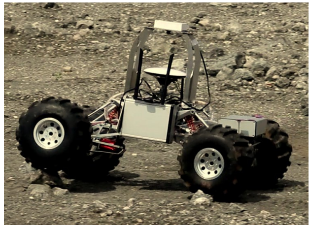
Figure 1: The AutoKrawler traversing uneven terrain in a lunar analogue site.
